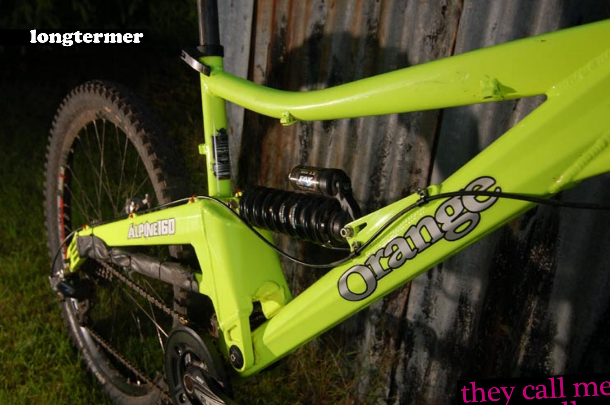
Due to the long stroke shock and high pivot the swingarm cross brace is necessary to maintain stiffness, it also makes a neat space to wrap an inner tube!
